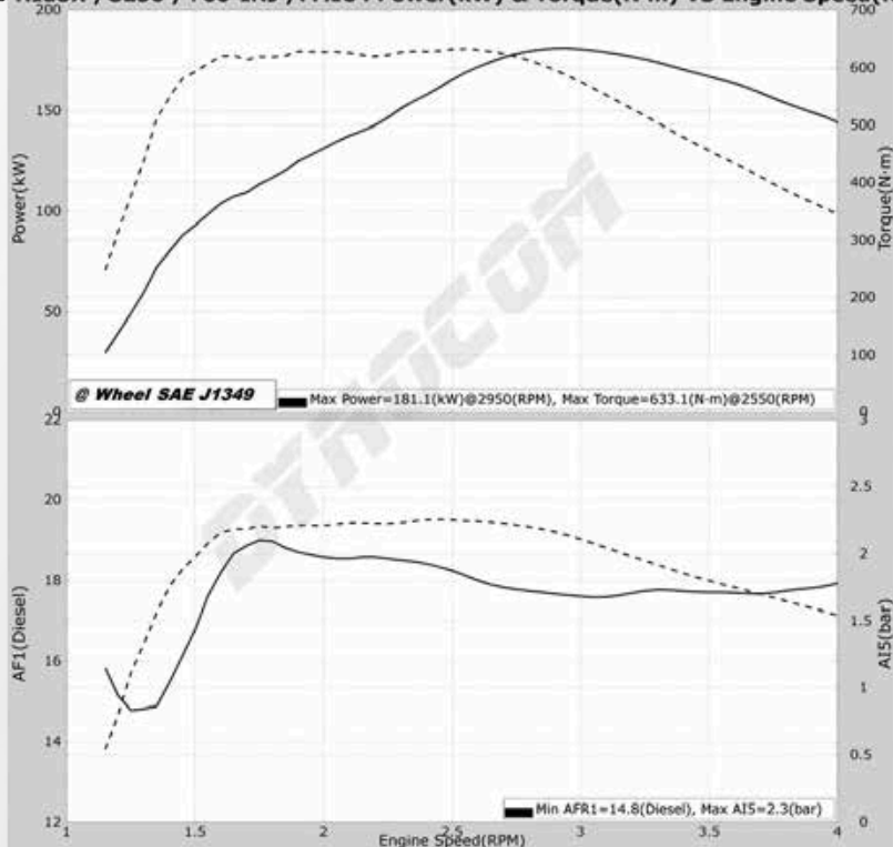
N70 HILUX /G250 /+60-INJ /FMIC : Power(kW) & Torque(N-m) VS Engine Speed(RPM)
