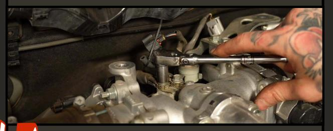
Ensure the bolts have clean, solid contact and that the battery is disconnected before attempting.
