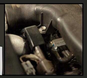
Using a 14 mm spanner, loosen and remove the 14 mm banjo bolt from the end of the fuel relief valve.
