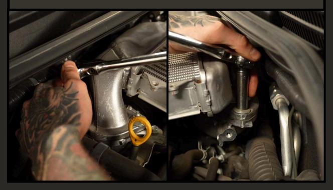
Remove the intercooler hoses. Once removed, block off the hose ends to prevent any foreign objects from entering the intercooler plumbing.
