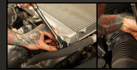
With a 12mm long socket, loosen the four intercooler mounting nuts in the pictures below.
