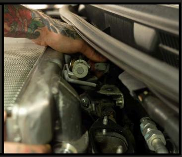
Lift the intercooler and disconnect the small pressure hose from the MAP sensor.
